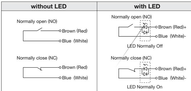
When using the switches with LED option, limit the current below 10mA.
